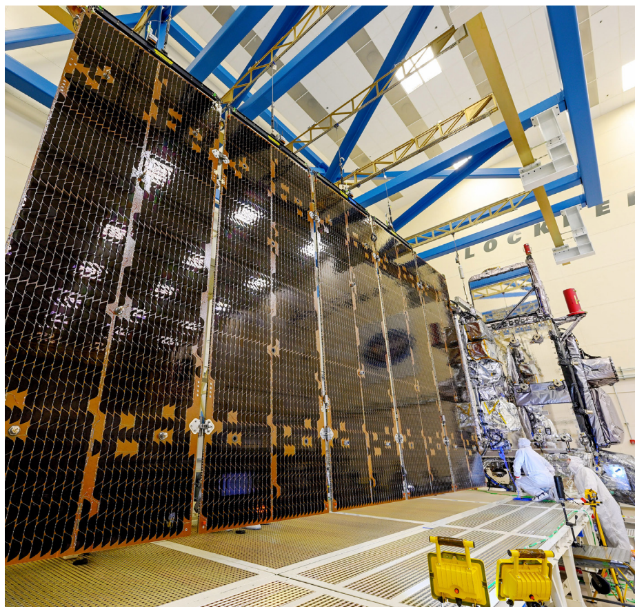
The GOES-U solar array fully deployed. Photo credit: Lockheed Martin
