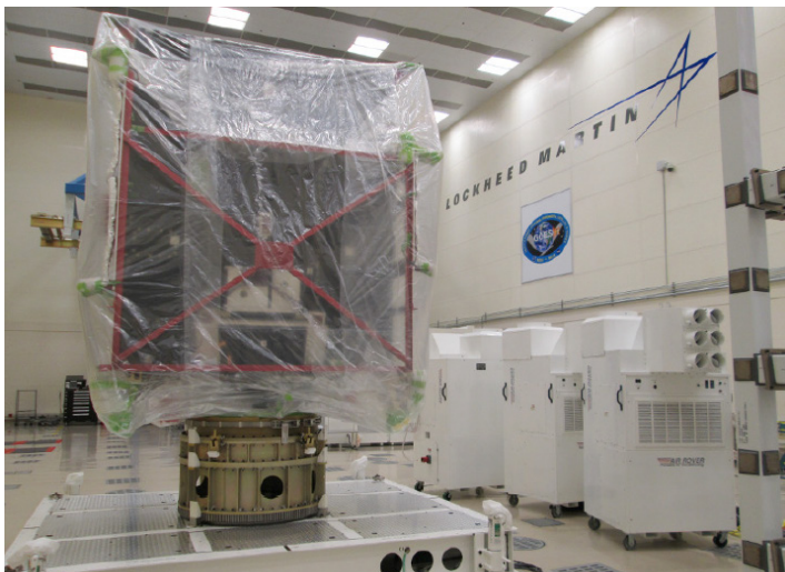
GOES-R satellite propulsion core module in the cleanroom at Lockheed Martin's Littleton facility. Credit: Lockheed Martin
