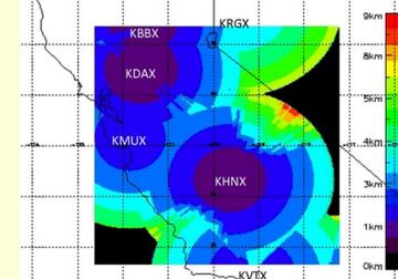
• A DEM and beam model were used to find locations where the radar beam intersects the terrain, similar to Lang et al. (2009), and correct for any partial occultation of the beam. For locations with >90% blockage, a higher available elevation angle was used.
