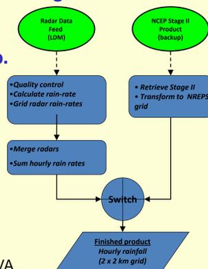
Figure 1: Layout of NREPS software system design for TVA.
