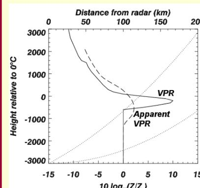
Figure 4. Model VPR (solid) and apparent VPR at 100 km range (dashed) used by NREPS in Central California. Also shown is the 3dB radar beam at 0.5° elevation (dotted).
