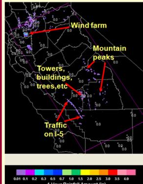
• To reduce the impact of non-precipitation in the radar data, methods devised by Steiner & Smith (2000) were employed as well as a "climatological" non-precipitation mask (areas that showed persistent rainfall during dry periods).
