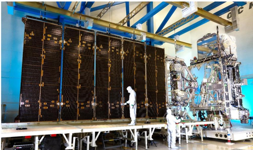
**Figure 11-3. The Solar Array installed on GOES-16**
