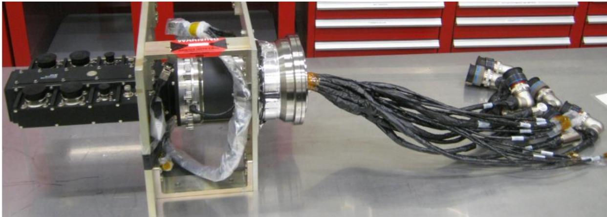
**Figure 15-6. Solar Array Drive/Slip Ring Harness Assembly**
