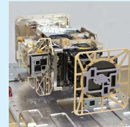
EXIS monitors solar irradiance in the upper atmosphere and detects solar flares that could interrupt communications and reduce navigational accuracy, affecting satellites, high-altitude airlines, and power grids on Earth. On board EXIS are two main sensors, the Extreme Ultraviolet Sensor
