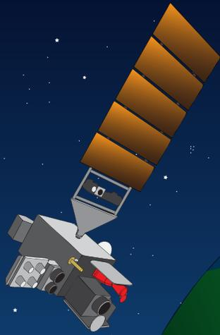
A new group of satellites called the GOES-R series should help us use information about lightning to warn of dangerous incoming weather. An instrument on the satellites, called the Geostationary Lightning Mapper (GLM), will detect both in-cloud and cloud-to-ground lightning, almost as soon as it happens. These lightning observations will help alert people to dangerous and intensifying storms and may lead to new and better ways to predict and prepare for severe weather!
