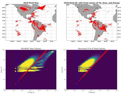
**Figure 1**. Sample during April 10, 2019 of raw GLM flashes (top left) and the distribution of flash area and energy for the flashes (bottom left). The right panels show quality-controlled data using an ABI Ch 13 brightness temperature threshold of -10°C, an energy threshold of 2x10<sup>-24</sup> J (blue line, bottom panels), and an area threshold equivalent to the function plotted that varies for a given energy (red line, bottom panels).
