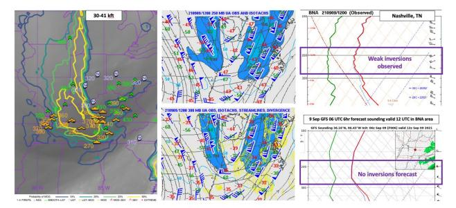
Figure 2. Left: CruiseNet 2.1 turbulence estimation product for 2 Sept 2021 1220 UTC. Contours indicate probability of turbulence and symbols represent pilot reports of turbulence; Middle: Corresponding GFS windfield; Right: Observed and GFS-modeled vertical transect in the area of turbulence.
