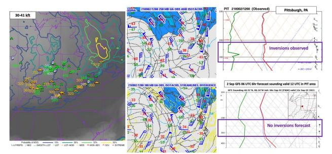
Figure 1. Left: CruiseNet 2.1 turbulence estimation product for 2 Sept 2021 1220 UTC. Contours indicate probability of turbulence and symbols represent pilot reports of turbulence; Middle: Corresponding GFS windfield; Right: Observed and GFS-modeled vertical transect in the area of turbulence.
