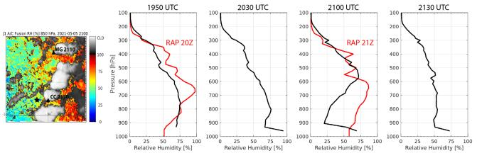
**Figure 4**. ABI/CrIS-NOAA20 RH fusion profiles at 1950 (NOAA-20 overpass time), 2030, 2100 and 2130 UTC at one selected location (40.48° N and 98.74° W, approx. 45 km west of Clay Center, is marked by a black star symbol in the left plot) are shown in black. The 2000 and 2100 UTC RAP RH profiles are shown in red.
