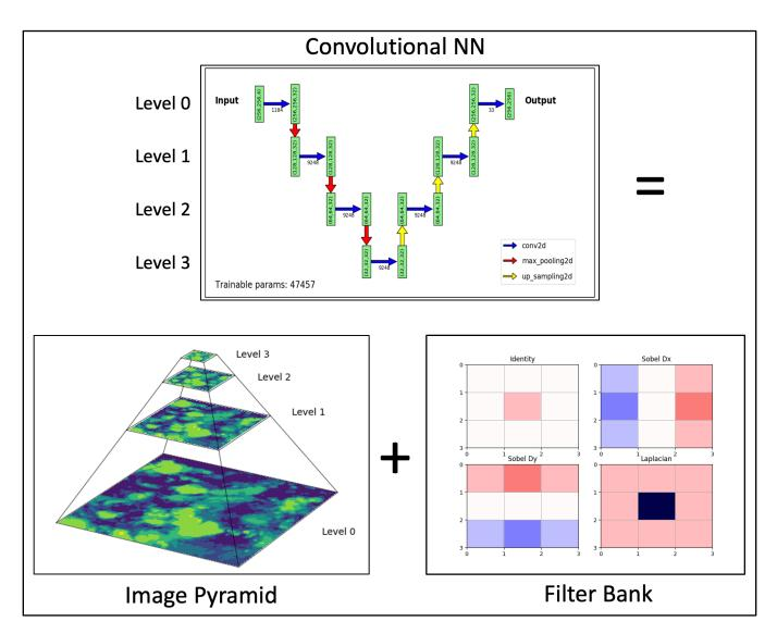
**Figure 1.** The GREMLIN convolutional neural network (top) can be represented as a combination of an image pyramid (lower left) and a filter bank of image kernels (lower right) with no loss in skill but far better interpretability than what is provided using Layerwise Relevance Propagation.
